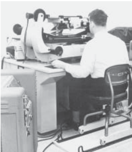
A mann stereo-comparator, used to measure objects in satellite reconnaissance photographs. This device was used to determine the height of the J-Vehicle, or N-1, on the launch pad. NPIC
