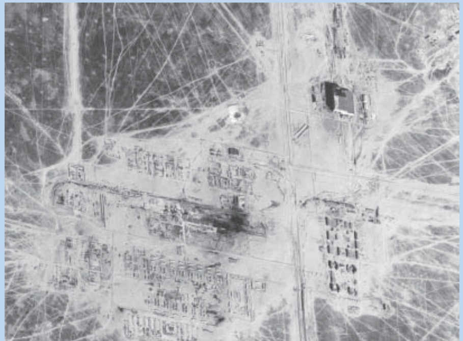
February 1966 KII-7 GAMBIT reconnaissance satellite photo of what the CIA designated Complex J at Tyura-Tam. The construction workers' barracks are at the lower left, the concrete batch plants are in the centre, the technical worker housing and technical facilities (Site 113 to the Russians) are at the right and the massive Missile Assembly Building (known to the Russian as the Assembly Test Building or MIK-112) is at the upper right.
