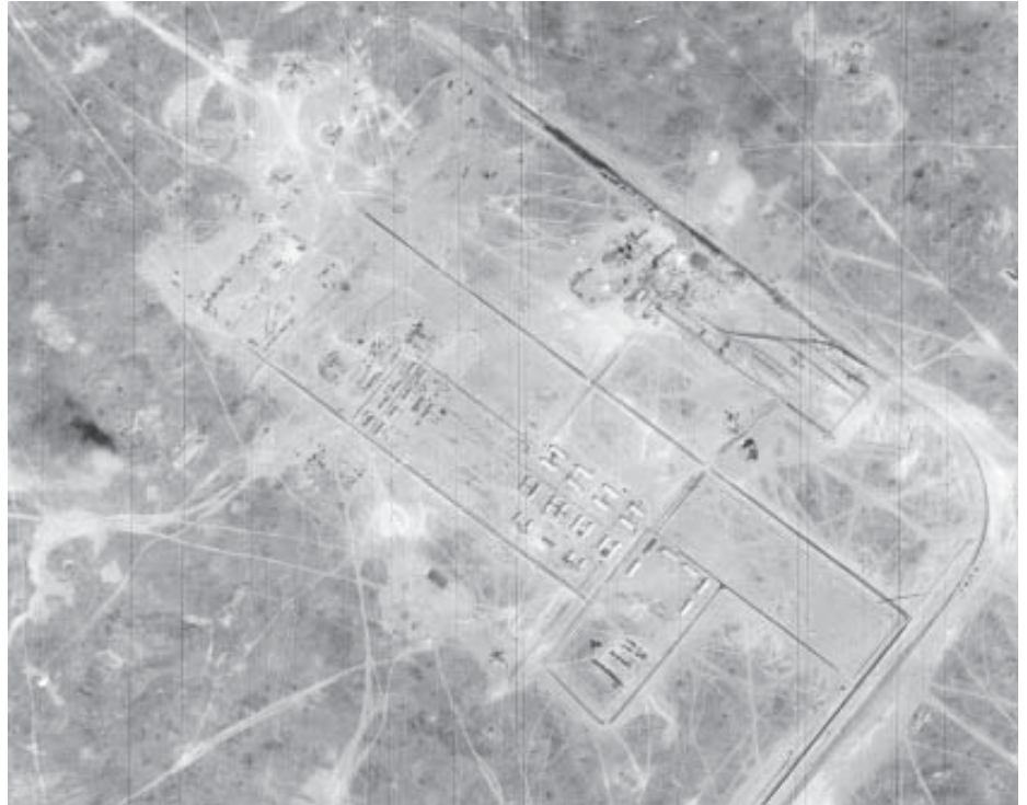
Summer 1963 KH-7 GAMBIT reconnaissance satellite photo of initial construction barracks at the Soviet N-1 launch facility. The buildings at bottom were for housing the construction workers. This was the first sign that a massive construction project was underway.
