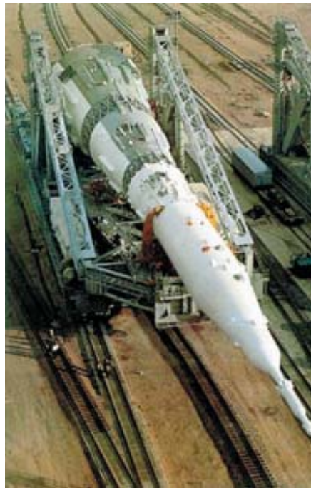
The first N-1 rocket is brought to the pad in early 1969. The form of the Transport-Installation Unit (TUA) with the N-1 give a definite impression of a giant grasshopper. files of Asif A. Siddiqi
