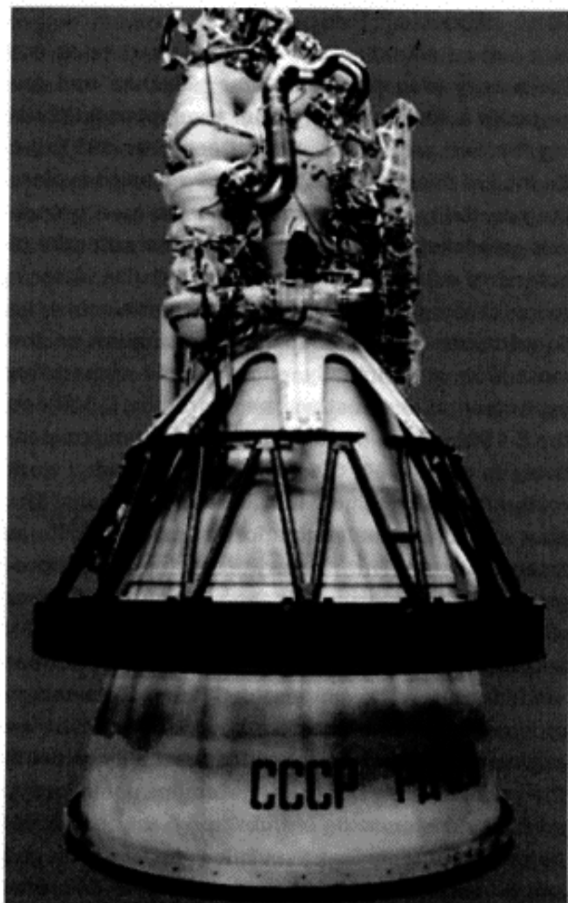
Fig 7. This is the RD-120 engine used on the second stage of the Zenit-2 booster. © Dietrich Haeseler
