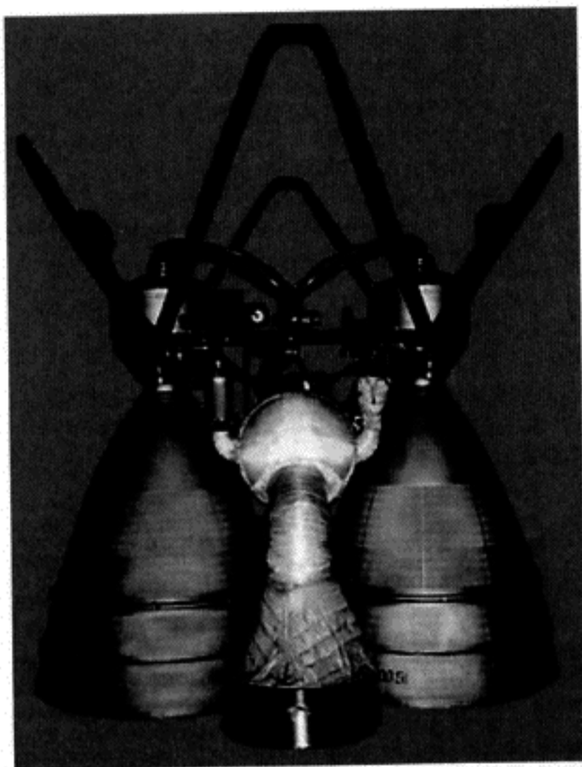
Fig. 3 Here is the RD-252 engine, used on the second stage of the R-36 (SS-9) ICBM. The RD-252 was essentially a high altitude version of the RD-250 engine, a two-chamber engine used as the 'base module' for all the engines on the R-36 ICBM developed in the 1960s. © Dietrich Haeseler
