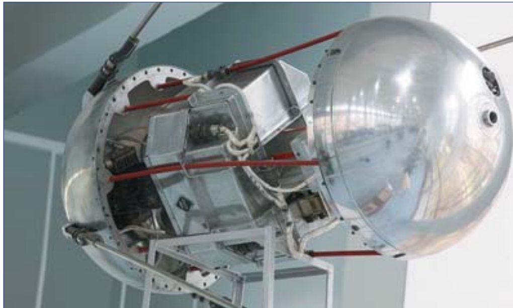
These images show an exploded view of the PS-1 satellite on display at the RKK Energiya Museum in Korolev outside of Moscow. Clearly visible in these images are the two casings of the satellite, the large battery package, and components of the radio transmitter. Seiji Yoshimoto/NPO InterCoS
