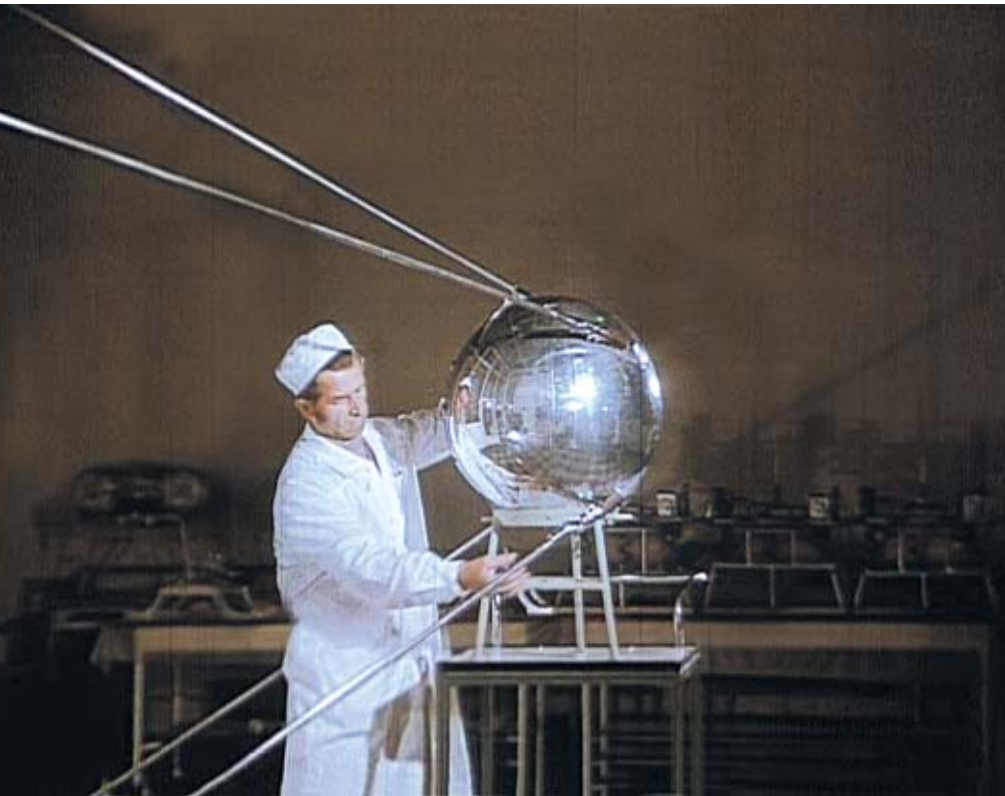
A still from a documentary on Sputnik shows a technician working on PS-1. More than likely this was a "re-enactment" staged soon after the Sputnik launch rather than the actual flight-model.
