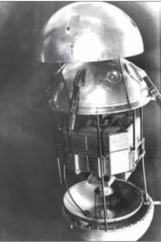
This exploded view of the PS-1 satellite clearly shows its constituent parts. From the top: the thermal shield, the "front" half-casing, the batteries, radio transmitter system, and the "rear" half-casing. National Air & Space Museum
